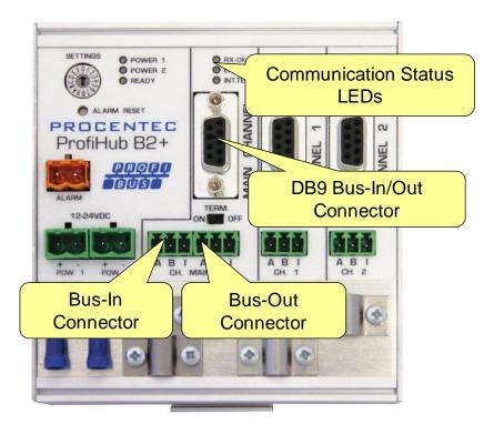
Fig. 13 - PROFIBUS DP backbone connection
