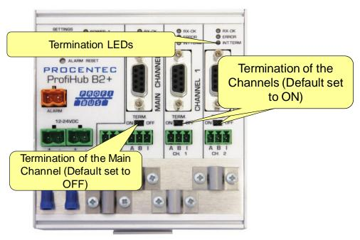
Fig. 15 - Termination Switches
