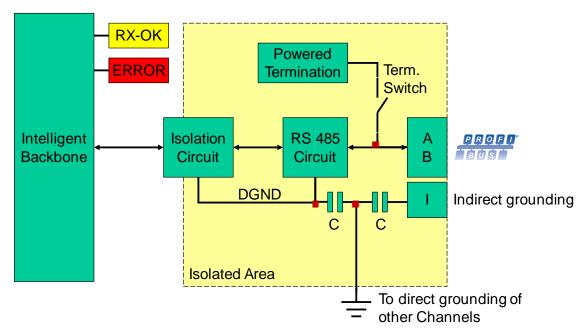
Fig. 5 - Channel structure
