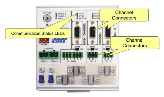
Fig. 14 - PROFIBUS DP spur connectors
