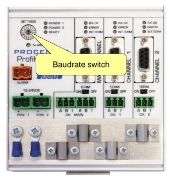
Fig. 16 - Baudrate speed switch
