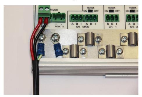
Fig. 12 – Connection to Ground Rail
