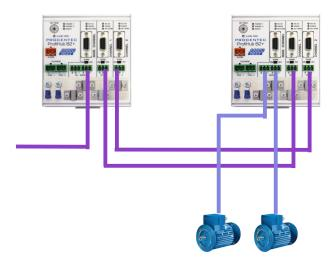
Fig. 17 - Redundant path between two ProfiHubs
